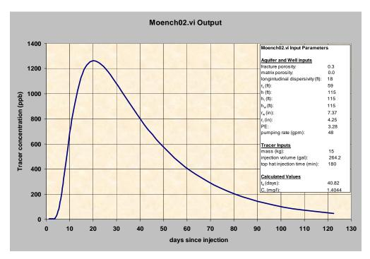
Figure 6. Prediction of Cross-Hole Conservative Tracer Testing in Screen #2 (q=48 gpm, PE=3.28)
