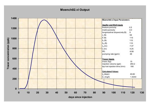
Figure 5. Prediction of Cross-Hole Conservative Tracer Testing in Screen #2 (q=48 gpm, PE=6.56)
