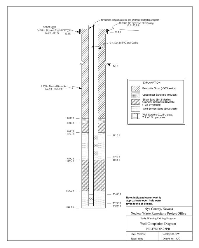
Figure 4. Completion Diagram for Well NC-EWDP-22PB
