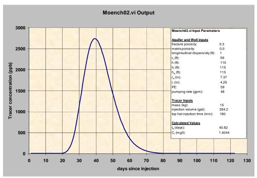
Figure 8. Prediction of Cross-Hole Conservative Tracer Testing in Screen #2 (q=48 gpm, PE=59)
