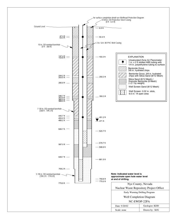
Figure 3. Completion Diagram for Well NC-EWDP-22PA
