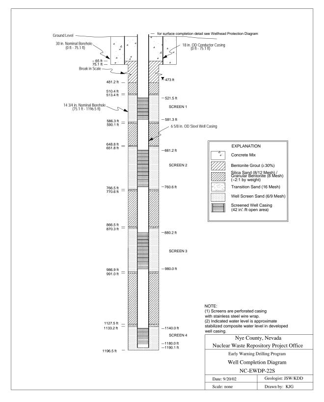
Figure 2. Completion Diagram for Well NC-EWDP-22S
