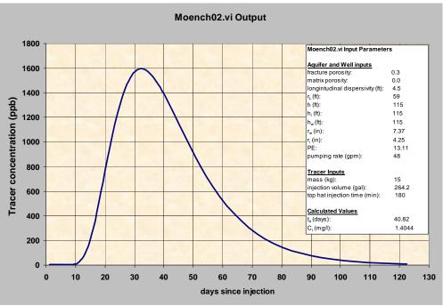
Figure 7. Prediction of Cross-Hole Conservative Tracer Testing in Screen #2 (q=48 gpm, PE=13.11)
