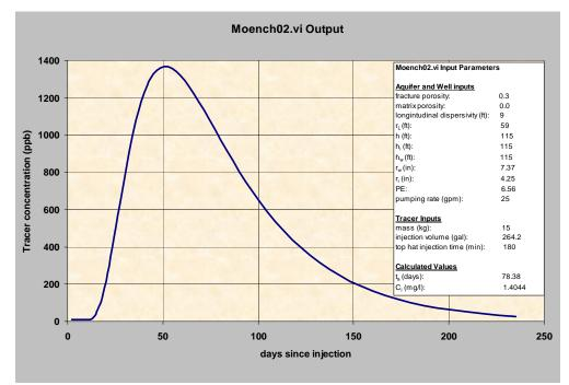
Figure 10. Prediction of Cross-Hole Conservative Tracer Testing in Screen#2 (q=25 gpm, PE=6.56)
