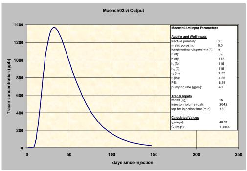
Figure 9. Prediction of Cross-Hole Conservative Tracer Testing in Screen #2 (q=40 gpm, PE=6.56)
