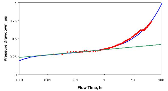
Fig. 4-Semi-log plot for Well 1-S, showing the semi-log straight line for permeability determination
