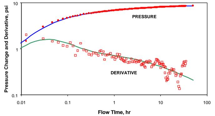
Fig. 5- Log-log plot for Well 3-D, with hemispherical flow as a negative half slope (-0.5) in the late derivative response
