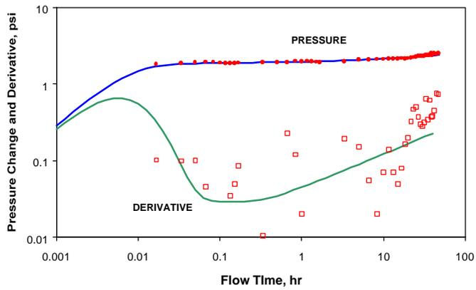
Fig. 8 - Log-log Plot for Well 9-SX, showing extended linear flow as +0.5 slope in the derivative curve at late times
