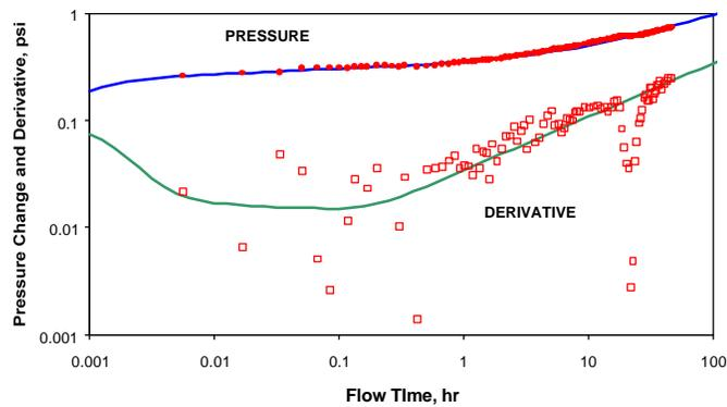
Fig. 3- Log-log Plot for Well 1-S, showing extended linear flow as +0.5 slope in the derivative curve at late times
