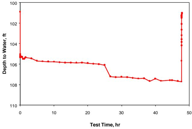
Fig. 7-Test response of Well 9-SX with anomalous 0.433 psi (1 ft) drop after 25 hr of flow
