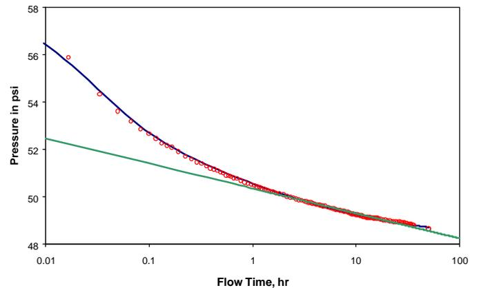
Fig. 6- Semi-log plot for Well 3-D. showing an erroneous semi-log straight line that should not be used for permeability determination
