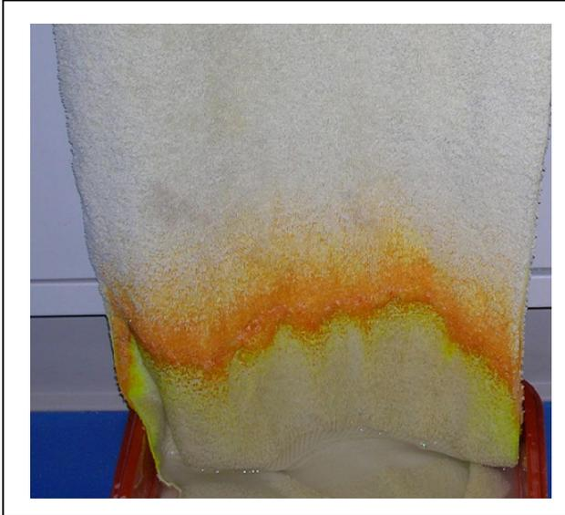
**Figure 4. Dye moves upward and concentrates in a towel dipped in water and dye. This is an example of the sequestration method presented, although in this case the evaporation is driven by the low-humidity room air rather than heat generation.**
