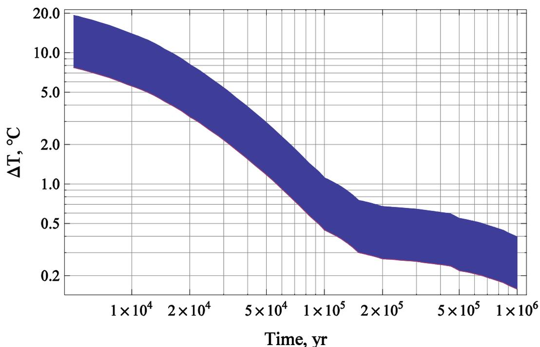
**Figure 7. Plausible temperature rise from outside to inside of the rubble formed as waste containers fail. This simple graph assumes a range of thermal conductivity characteristic of soils.**
