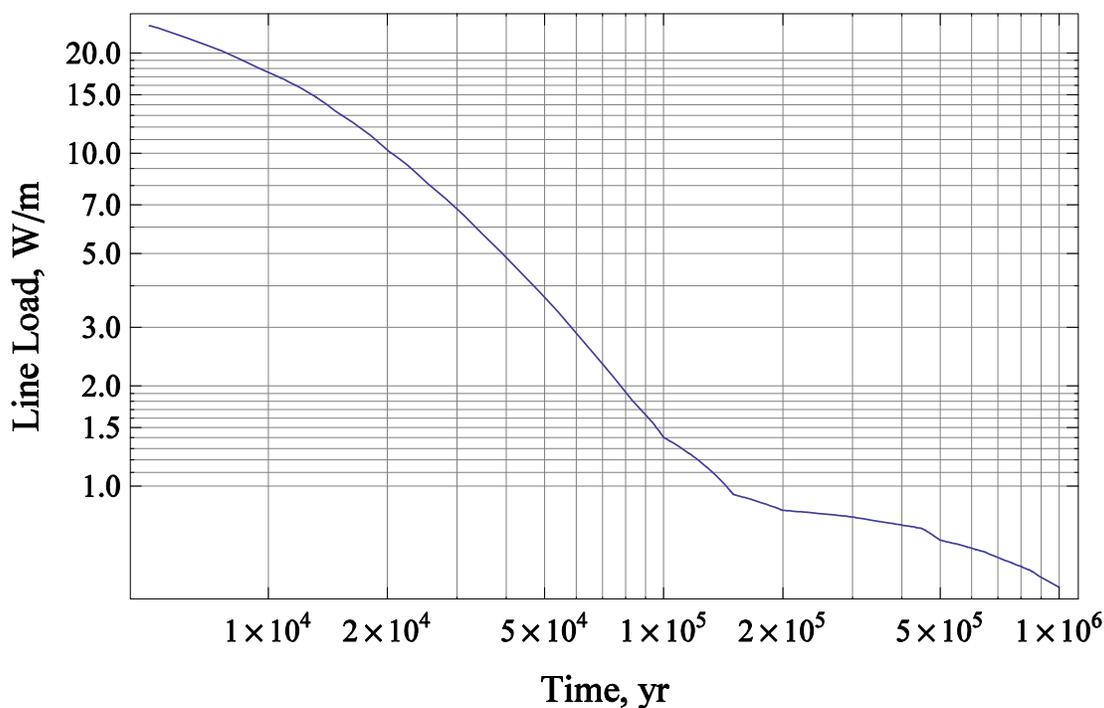
Figure 6. Line load on a logarithmic scale. Small but significant heat release occurs beyond one million years.
