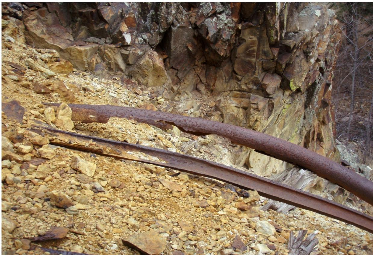
**Figure 1. Example of general corrosion that is non-uniform. North Percha Creek mine, New Mexico.**
