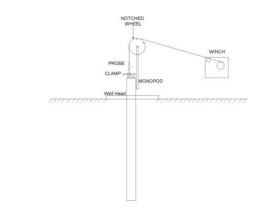
Figure 1. Setup of Notched Wheel, Probe, Clamp, Monopod, and Winch at Well Head
