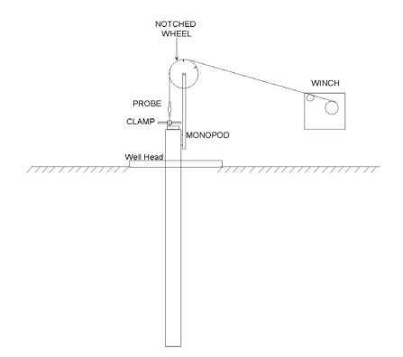
Figure 1. Setup of Notched Wheel, Probe, Clamp, Monopod, and Winch at Well Head
