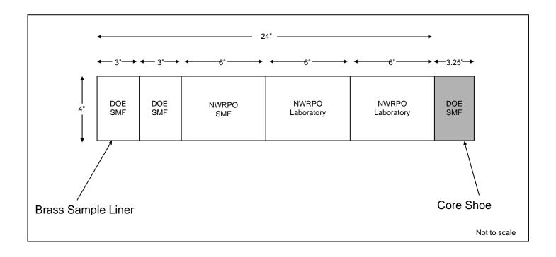
Figure 5 Distribution of Core Segments in 2.0-foot Core Barrel
