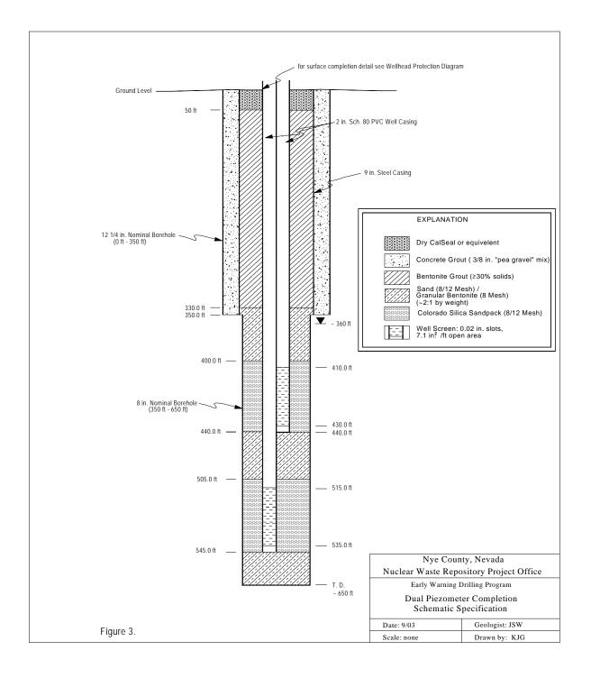
Figure 3 Dual-Piezometer Subsurface Completion Diagram
