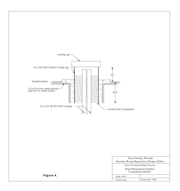
Figure 4 Dual-Piezometer Surface Completion Diagram
